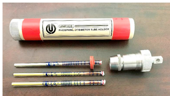
Fig. 2. Protective PVC tube, red rubber grommets, and aluminum caps for holding dosimeter glass tubes while deployed in commodities and three dosimeter tubes which were exposed during fumigation trials. (For interpretation of the references to color in this figure legend, the reader is referred to the Web version of this article.)
